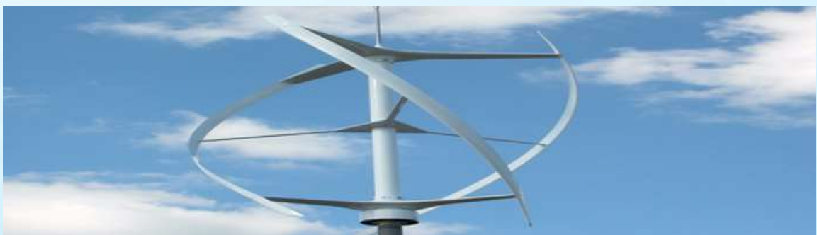
Vertical Axis Wind Turbine
